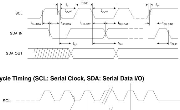
Write Cycle Timing (SCL: Serial Clock, SDA: Serial Data I/O)
