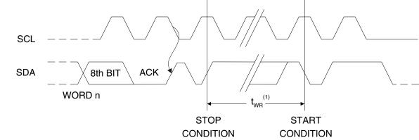
1. The write cycle time  $t_{WR}$  is the time from a valid stop condition of a write sequence to the end of the internal clear/write cycle. Note:
